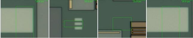
Fig. 2. Optical inspection of resistor layer structures revealed no unlifted sputtered NiCr thin film after lift-off.
