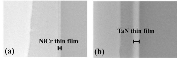
Fig. 4. Thickness measurements of (a) NiCr and (b) TaN thin films with identical inline sheet resistance on GaAs substrates.
