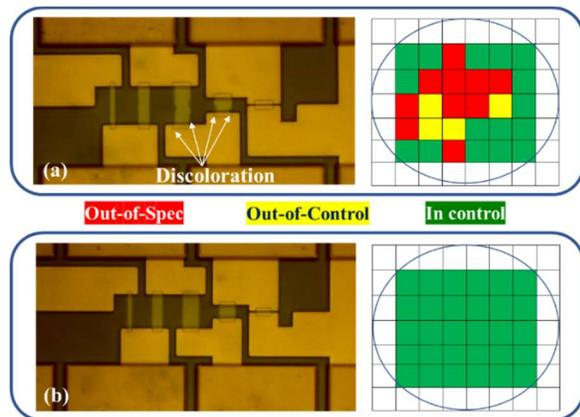
Fig. 8. Optical inspection of resistor TLM structures for (a) NiCr and (b) TaN product wafers. Sites affected by discoloration had Out-of-Spec (OOS) or Out-of-Control (OOC)  $R_s$  as indicated by the color-coded wafer maps.
