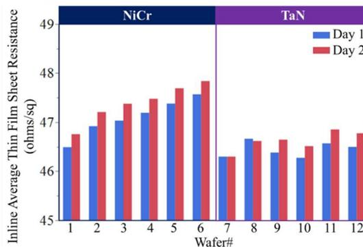
Fig. 7. Oxidation effect on R<sub>s</sub> in the ambient environment
