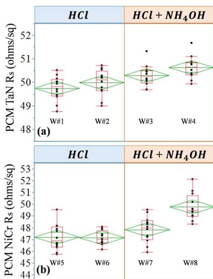
Fig. 5. DOE of pre-cleans using HCl and NH<sub>4</sub>OH prior to the sputter deposition of (a) TaN or (b) NiCr.
