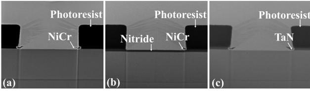
Fig. 1. FIB cross section of resistor layer's negative resist profile after sputter deposition for (a) NiCr with DAL etch, (b) NiCr without DAL etch, and (c) TaN with DAL etch.
