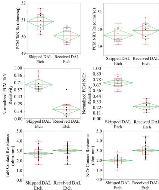
Fig. 3. The effect of DAL etch on  $R_s$ , resistivity, and contact resistance for TaN and NiCr.
