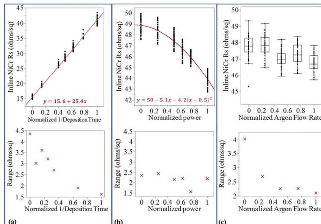
Fig. 6. Inline NiCr R<sub>s</sub> has a (a) linear relationship with 1/deposition time, (b) quadratic relationship with power, and (c) negative correlation with argon gas flow rate.
